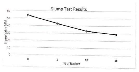
The above fig shows the slump results. It was observed that, the slumps decreased as the rubber content were increased in the mix. It was a Low Slump (25 - 50mm). It was suitable for Low Workability mixes used for foundations with light reinforcement. Roads vibrated by hand operated machines.
